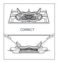
Figure 22 Correct placement of wok stand
